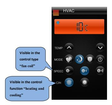
The HVAC control interface is shown as the picture at left. In the case of different control functions and control types, the operation interface will be different.
