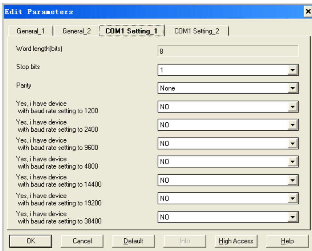
Fig. 4.2 Parameter window "COM1/2 Setting" (1)
